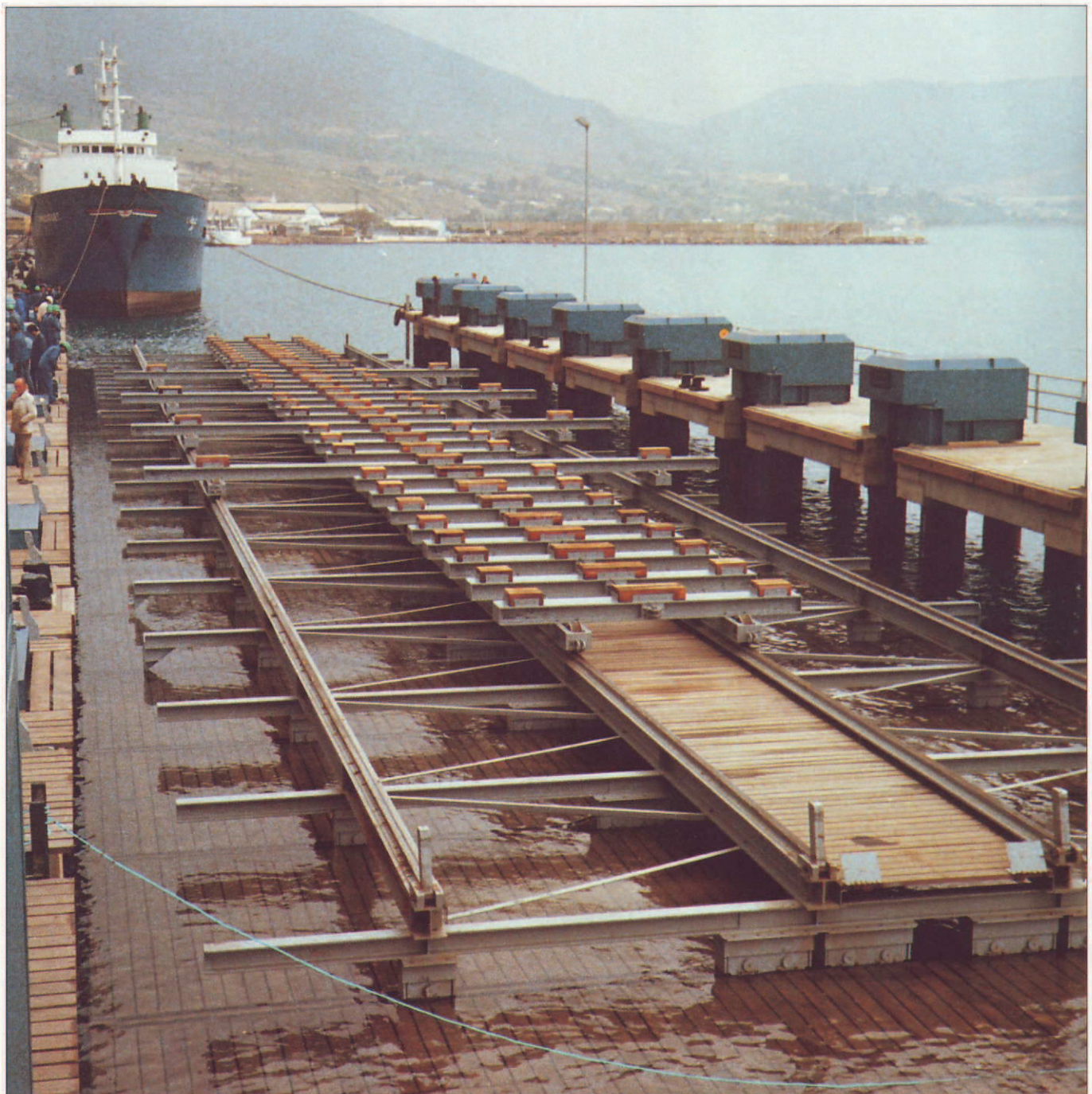
LIFT-DOCK and transversal transfer carriage for 6500 tons nominal lifting capacity (NLC)
