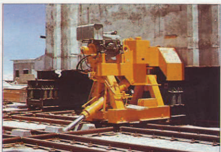
Schies-Defries mover units and heavy duty wheel sets for caisson transfer
