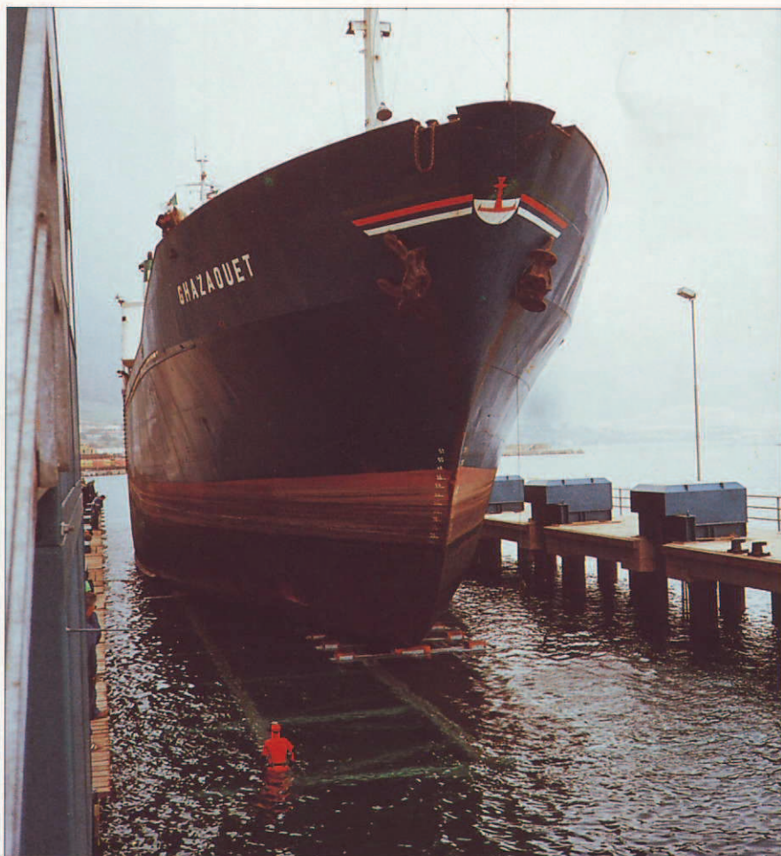
Cargo vessel with 12,000 DWT in launching process on a lift-dock®
